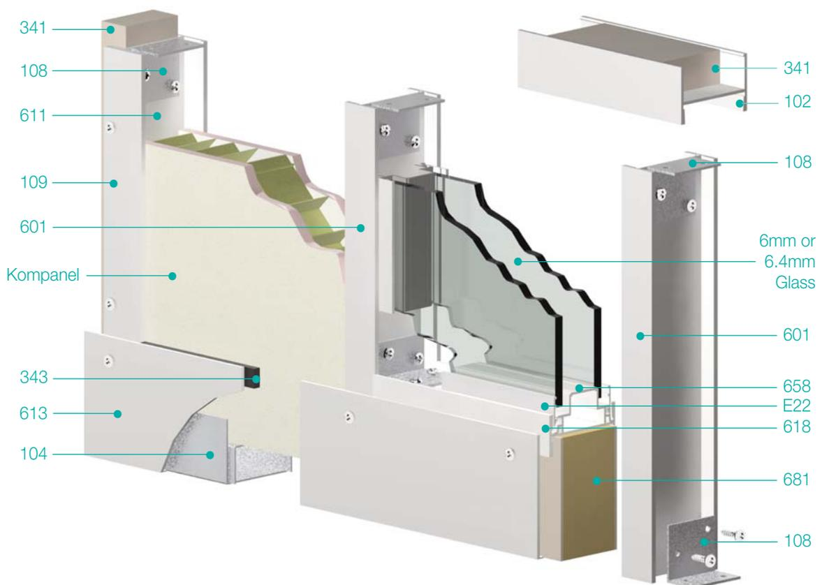
50mm Aluminium framed composite system with vertical posts variations for height up to 6 metres
