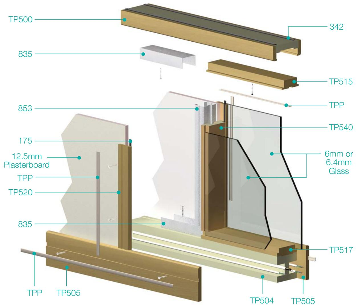
75mm Steel stud system with radius veneered cover trims
