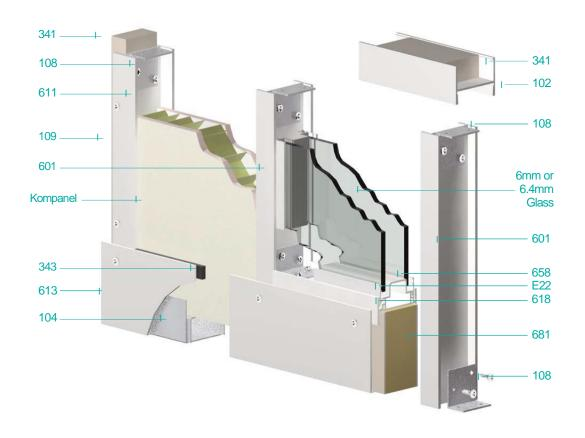
50mm Aluminium framed composite system with vertical posts variations for height up to 6 metres
