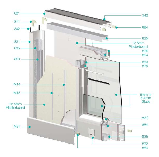
75mm Steel stud system with radius aluminium cover trims
