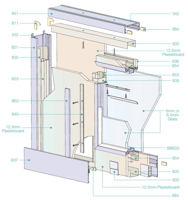
75mm Steel Stud & Plasterboard Partitioning System with Square Aluminium Cover Trims
