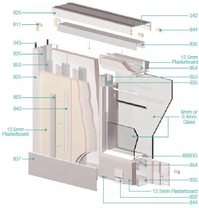
100mm Steel stud & double board system with square aluminium cover trims
